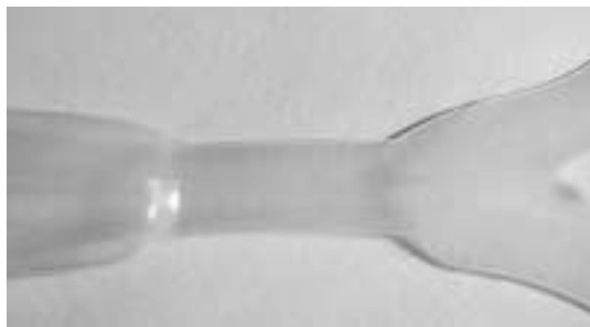
Figure 1.17: Necking and drawing in a 6-pack holder.
