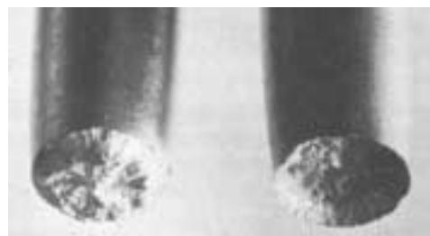
Figure 1.15: Cup-and-cone fracture in a ductile metal.
