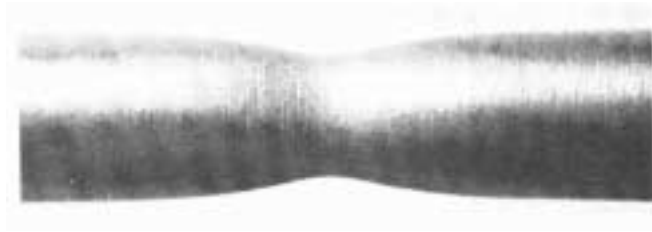
Figure 1.14: Necking in a tensile specimen.
